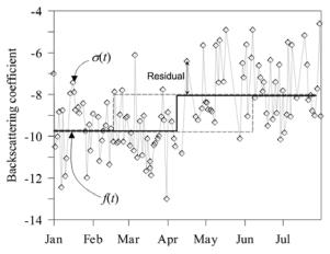
Figure 3. Concept of fitting of piecewise step function to GM normalized backscatter time series.
