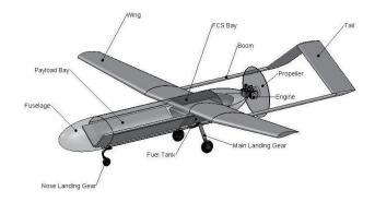
Figure 1. Josaphat Laboratory Experimental UAV (JX-1)
