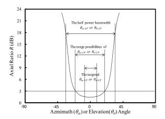
Figure 3. The 3-dB AR beamwidth illustration
