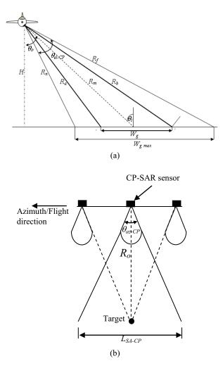
Figure 5. UAV CP-SAR geometry system: (a) slant range view and (b) azimuth plane view
