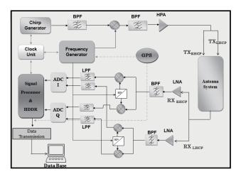
Figure 4. UAV CP-SAR sensor circuit design
