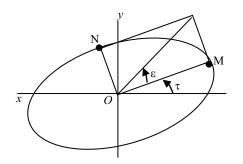
Figure 2. Electromagnetic Wave Polarization Parameters
