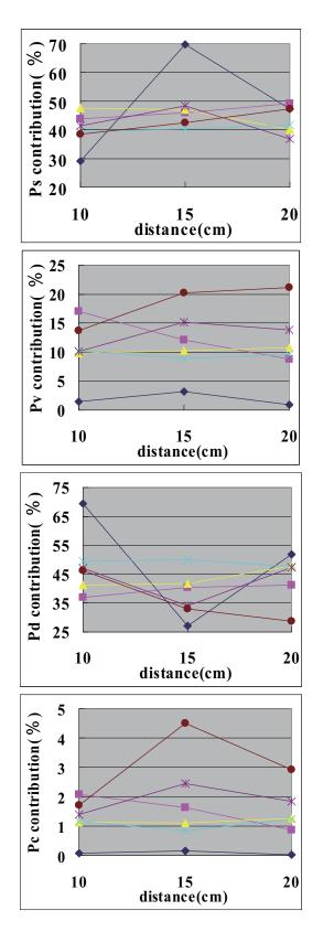
Figure 6. Relationship between four-components and the distance of the blocks. From upper to lower, surface scattering, volume scattering, double bounce scattering, and helix scattering are shown, respectively.
