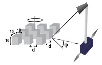
Figure 2. Schematic diagram of the measured structure. d is the distance of the blocks (three distances),  $\phi$  is the slant angle of the blocks (six angles).
