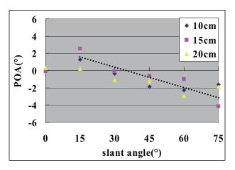
Figure 3. Relationship between POA and the slant angle of the blocks.
