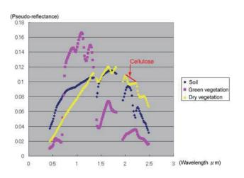
Figure 3. Cellulose absorption
