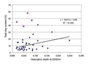
Figure 11. Relationship between total clay content and the absorption depth at 2200nm of reflectance (uncorrected)
