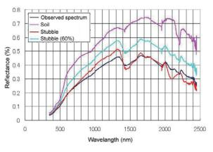
Figure 7. Reflectance obtained in the area with shadow effect of stubble
