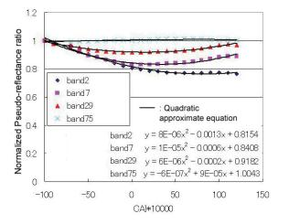
Figure 5. Correction curve using the normalized pseudo-reflectance
