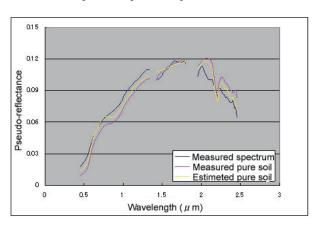
Figure 9. Estimated pure soil spectrum and measured pure soil spectrum
