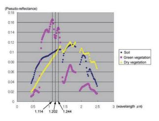
Figure 2. Water absorption in vegetation seen around  $1.2 \,\mu$  m
