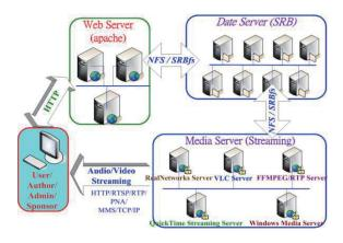
Figure 5. Illustration of the schematic view of stream servers, and storage pool
