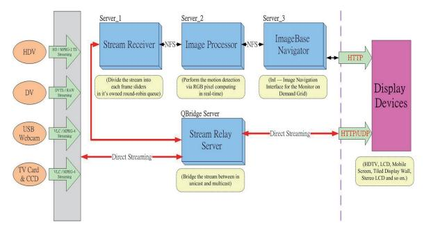
Figure 1. Architecture blocks and stream pipeline
