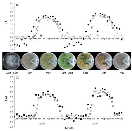
Figure 2. Time series of *in situ* LAI against estimated LAI based on (a) MODIS NDVI and (b) MODIS EVI. The signs of cross, open signs and solid sing are *in situ* LAI, LAI based single relationship and LAI based double relationships, respectively, from 2005-2006.
