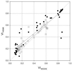
Figure 3. Comparison between *in situ* NDVI (solid circle) and EVI (open rectangular) from hemispherical spectroradiometer with NDVI and EVI from MODIS (solid circle).
