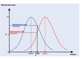
Figure 9. Membership of a class according to the principle of fuzzy logic.
