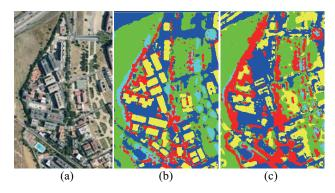
Figure 5. Aerial image for reference (a), results of SVM classifications with LIDAR (b), and without LIDAR (c)
