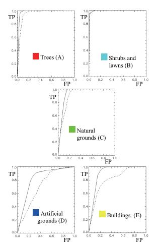
Figure 8. ROC curves in the SVM classifications with (straight line) and without (dotted line) LIDAR. TP and FP are true positive and false positive
