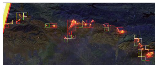
Figure 5: Fire detection result. Red:Fixed test Green:Contextual test under 1000\text{m} resolution Yellow:Contextual test under 250\text{m} resolution
