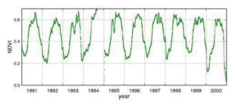
Figure 3. An example of NDVI time series from 1991 to 2000. This time series is composed of daily mean NDVI (8-km resolution) over the land areas of Japan derived from NOAA/AVHRR observation. Daily NDVI values were derived by the temporal window operation (Suzuki and Kondoh, 2005).
