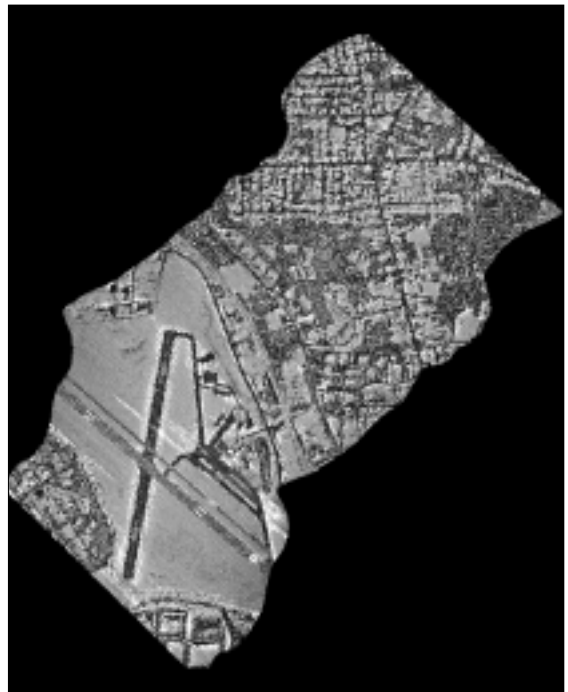
AeroScan LIDAR intensity image (white = high received signal, black = low received signal).
