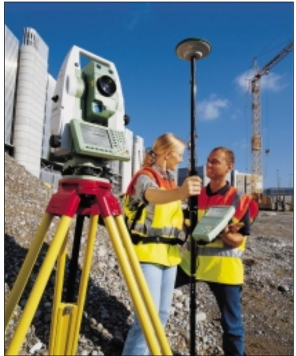
*GPS and TPS stations working together for the first time in history. The new Leica Geosystems Universal System 1200 GPS and TPS survey stations offer standardised operation through identical user interfaces with graphic display and consistent data management.*
