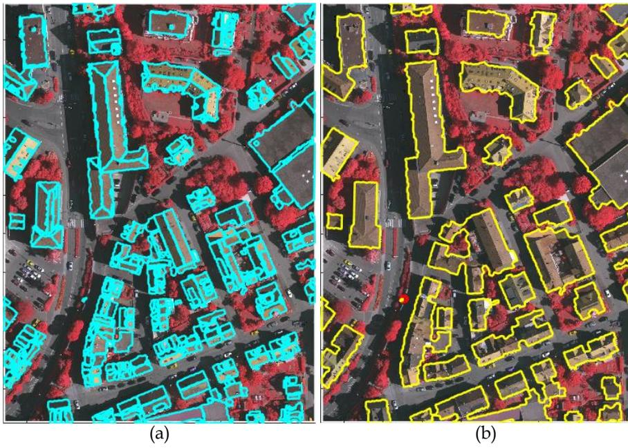
Figure 2: (a) Extracted plane boundaries, and (b) Extracted building boundaries. Both are laid on the for the ISPRS (Area 1) image just for demonstration
