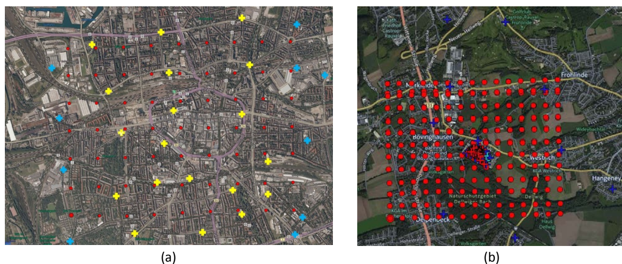
Figure 2: Collected GCPs in the City center and in Museum area – Zeche Zollern (not all the collected points are displayed in the image)
