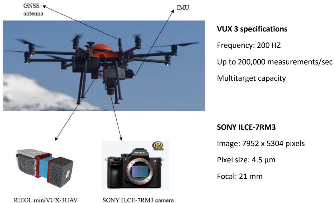
Figure 1 – The used drone and technical specifications of the payload
