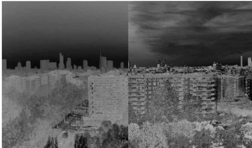
Figure 2: Comparison of saturation channel images: the left panel shows a clean-air scene, whereas the right panel depicts a polluted scene associated with high PM 2.5 concentration.
