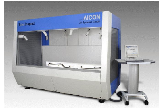
Multi-camera measurement system AICON (2006)
