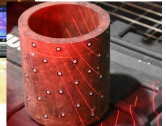
Laser projection Creaform HandyScan
