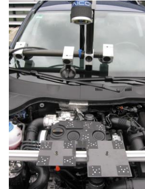
High speed 6DOF measurement
