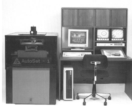
Digital image comparator GSI AutoSet-1 (1986)
