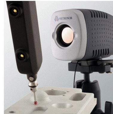
Tactile mono system Metronor (2002)
