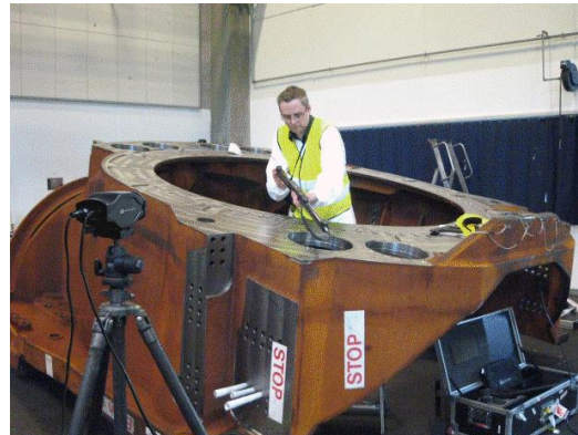
Multi-camera probing by intersection
